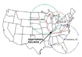
Triangulation is a method that uses distance information determined from 3 seismic stations to uniquely locate the earthquake. On a map, circles are drawn around each seismic station. The radius of the circle are scaled to the estimated distance from the station to the earthquake. The 3 circles will share one unique intersection that locates the earthquake.
