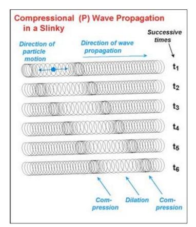
Compressional (P) wave propagation in a slinky. A disturbance at one end results in a compression of the coils followed by dilation (extension), and then another compression. With time (successive times are shown by the diagrams of the slinky at times t1 through t6), the disturbance propagates along the slinky. After the energy passes, the coils of the slinky return to their original, undisturbed position. The direction of particle motion is in the direction of propagation.
