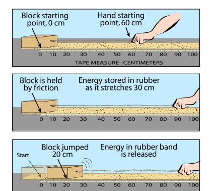
Basic "earthquake machine". Hand represents the regional force acting on the plate which, in this case, pulls on a rubber band. The force applied is proportional to the length of the rubber band.
